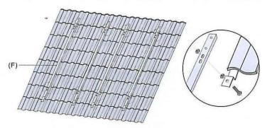
B. To fix the collectors track (F) on the mounting sheets.
