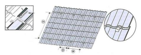
A. to fix the mounting sheets at the roof, ( the size (H), (W) please check the FORM 1,)
