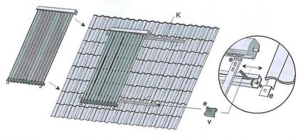
B. To fix the runner tracks (K), optional parts at the mounting sheets, the collectors mounted by the runner screws.
