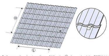
A.to fix the mounting sheets on the roof,( the size  $\widehat{\mathbb{H}}$  please check the FORM 1,) the  $\widehat{\mathbb{L}}$  length not longer than the width of collectors.
